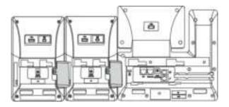
Connect the USB jack on the host phone and the mini USB jack on the expansion module using one supplied cable.
