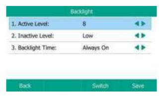
2. Press ( ) or ( ), or the **Switch** soft key to select the desired level from the **ActiveLevel** field on the host
