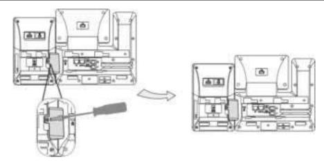
If you want to connect two or more expansion modules, pull out the silica gel and connect two expansion modules as shown below.
