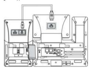
**Note:** Power is automatically transferred from the host phone to the expansion module(s) upon connection. If you want to use more than one expansion modules on a single phone, you need to connect an additional Yealink power adapter (5V/2A) to any one of the expansion modules
