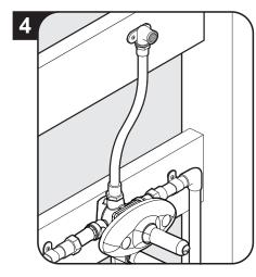
Determine shower location. Install crossbeam and secure a 90° elbow with hardware (not included). Connect elbow to tee.
