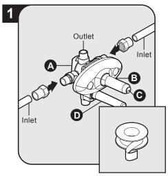
Connect hot and cold valves using 1/2" copper adapters and lines. **Note:** Supply lines not included. DO NOT apply heat directly to valve bodies.
