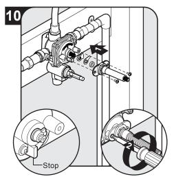
Reposition mechanical stop so that it is on the right side of the valve cover stop. Reattach stem assembly.
