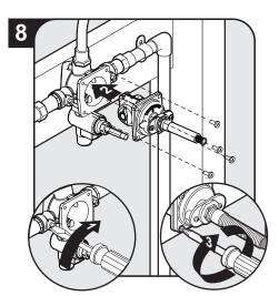
Close integral stops. Reinstall stem assembly, valve cover and cartridge in same configuration. Pressure test valve. *Note: Water pressure must be applied to both hot and cold inlets at the same time.*
