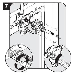
Remove stem assembly, valve cover and cartridge as one unit. Open integral stops to flush supply lines.
