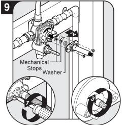
If water drips from outlet, remove stem assembly, mechanical stops and washer. Rotate cartridge stem clockwise until it stops.
